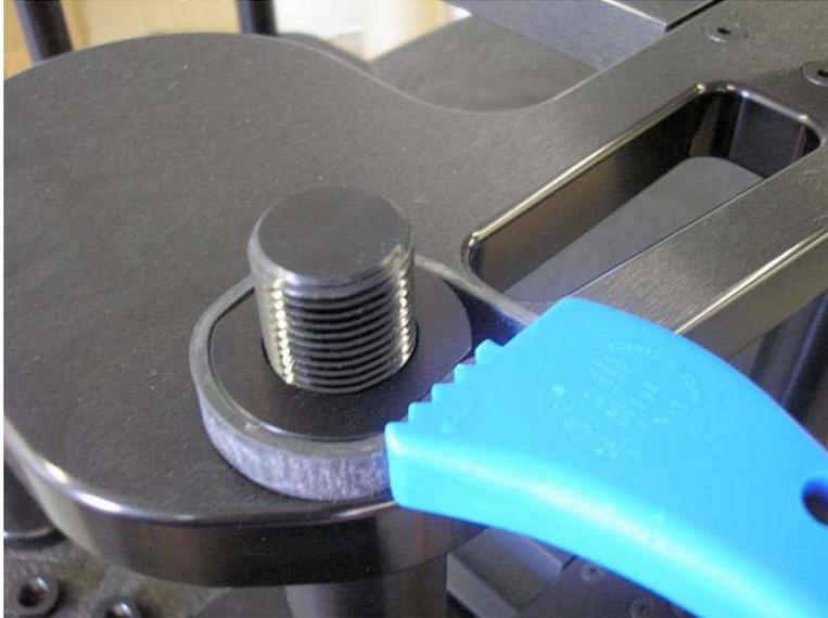
**Step 12.** *Screw the Locking Nut onto the threads of the struts completely as shown in Photo 13. Screw it all the way down until the Washer comes in contact with the Locking Nut. Light hand tight is fine. Do not put a large torque on Washer.*
